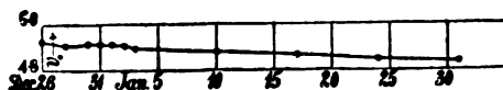
Fig. 36.—Chart showing loss of standard volumes of gas in diver in lapse of days. Diffusion of air through \text{AlCl}_3 solution.
